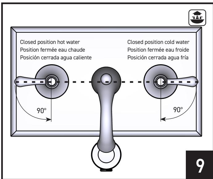
1. Rotate handles until they are aligned in the proper closed position.
